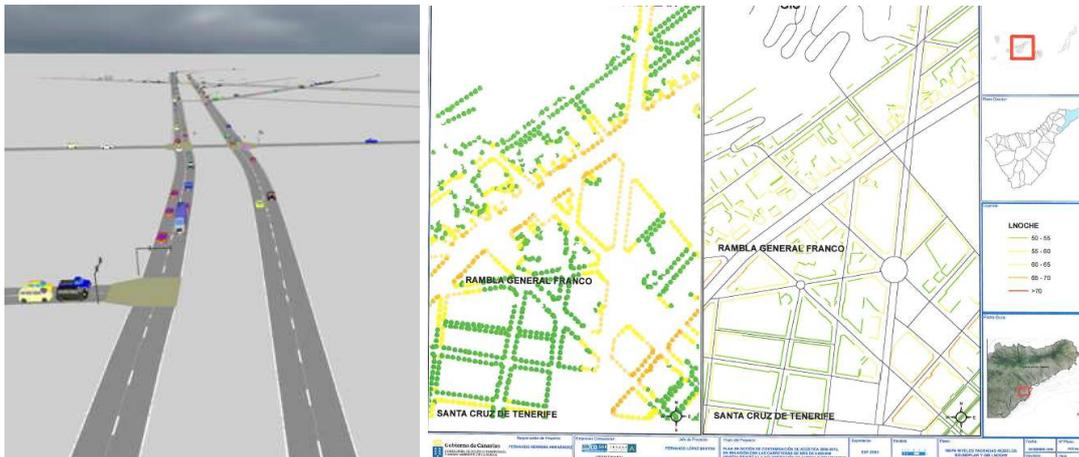
Figure 7 – Traffic microsimulation of La Rambla and surroundings during night hours. Current detailed noise exposed maps are developed based in the output of this traffic model.
