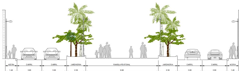
Figure 6 – Cross section of La Rambla.
